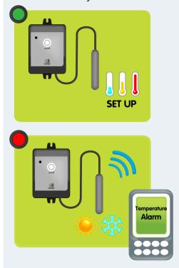
The Mobeye ThermoGuard runs entirely on batteries for more than a year. Upon a low battery voltage it will send a notification. When using an external power supply (12 VDC or mains), it can also send "power failure" notifications. It has two additional inputs. By connecting an external sensor all kinds of situations can be monitored, such as a machine process or the closing of a door.
