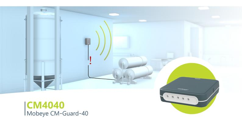
The Mobeye CM4040 is a universal alarm detector with four potential-free inputs and built-in communication module. It serves to monitor various sensors and control technical installations. NO/NC contacts can be connected to the inputs. A status change triggers an alarm or recovery message. The detector operates on the 2G and 4G LTE-M network.
