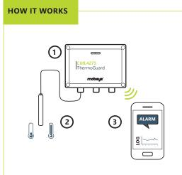
The Mobeye CML4275 continuously measures the temperature values and logs these periodically. In this way you are fully informed about alarm situations and the complete temperature trend.
