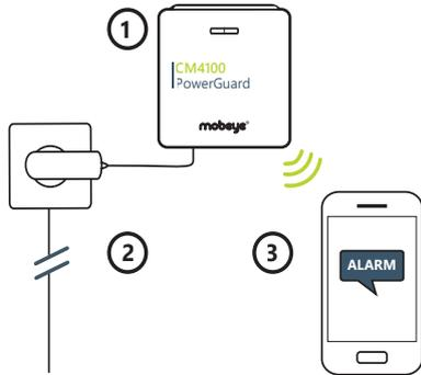
The Mobeye CM4100 monitors the availability of the external power and the status of connected fault contacts. The alarm dialer immediately sends a notification when the status changes. This means you are always well informed.
