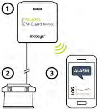
The Mobeye CML4055 monitors the voltage value of a connected battery or analog sensor. It measures the values continuously in order to instantly alarm in the event of deviations, and logs them periodically.
