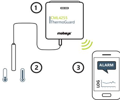
The Mobeye CML4255 continuously measures the temperature values and logs these periodically. In this way you are fully informed about alarm situations and the complete temperature trend.
