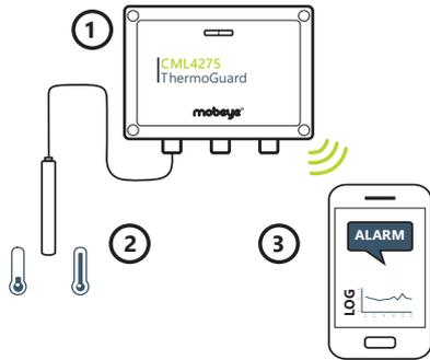
The Mobeye CML4275 continuously measures the temperature values and logs these periodically. In this way you are fully informed about alarm situations and the complete temperature trend.
