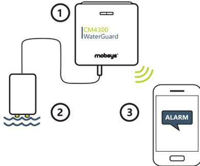
The Mobeye CM4300 monitors whether a room is dry. In the event of a water leak, it immediately sends a notification. This way you will detect a water leak in time and prevent water damage.
