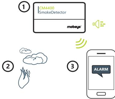
The Mobeye CM4400 smoke detector kit warns people on the spot in the event of a fire, as well as contacts elsewhere. It makes the difference in helping the vulnerable and in the event of fire in vacant buildings.
