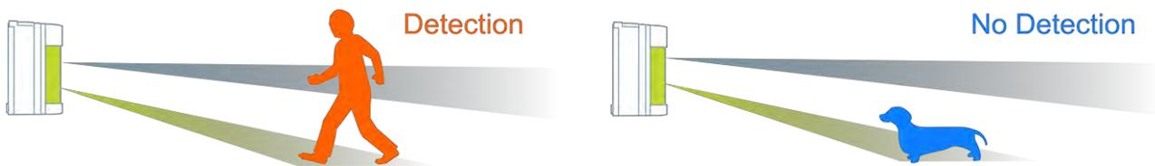
Alarm when both sensors detect movement.
