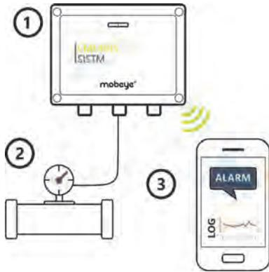
The Mobeye SISTM measures the analog sensor values. Any sensor with a suitable output signal can be connected. If there is no voltage on site, the SISTM measures, reports and logs completely autonomously.
