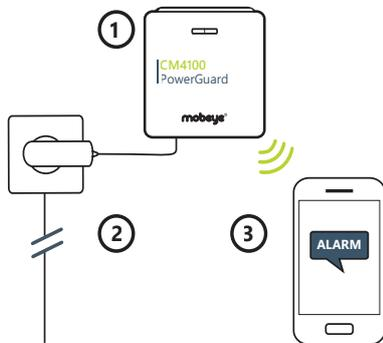
The Mobeye CM4100-G monitors the availability of the external power and the status of connected fault contacts. The alarm dialer immediately sends a notification when the status changes. This means you are always well informed.
