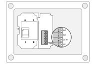
As default the input is programmed as Normally Open (NO) contact. This means the input is triggered if the input is closed for at least 1 second. In case the contact is Normally Closed (NC), see paragraph 5.10. If the sensor needs to be activated for a longer period before triggering an alarm, see 5.10.
